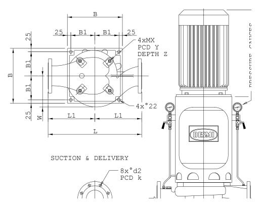
Manometer: 1/4" BSP. Drain: 3/8" BSP. Priming: 1/2" BSP
