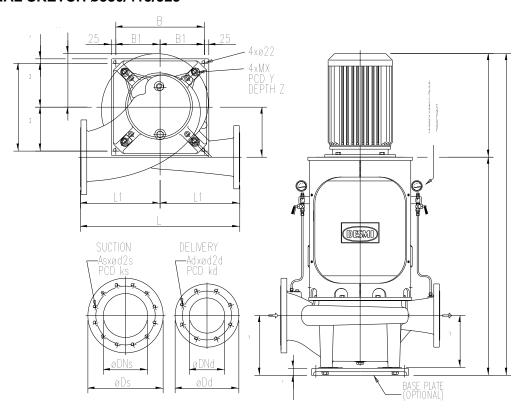
Manometer: 1/4" BSP. Drain: 3/4" BSP. Priming: 1/2" BSP
